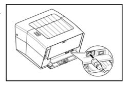
2 Connect the other end of the power cord to a power outlet.
